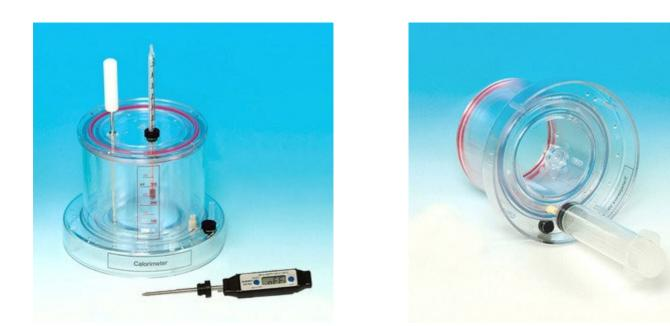
Before the beginning of the experiment, remove air from the air space inside the calorimeter with a syringe (the right picture or movie).
