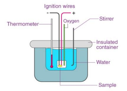
Calorimeter: A laboratory apparatus used for measuring the quantity and direction of heat flow
